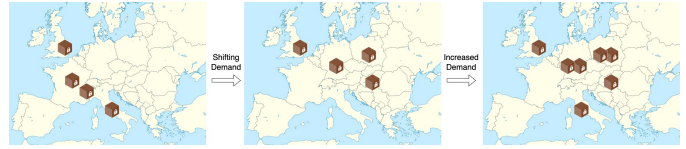
Fig. 1. Illustration of dynamically changing redundancy and fragment placement based on real traffic
